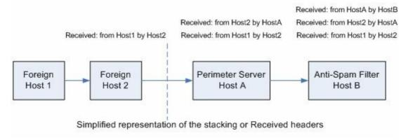
Here the spam filter (Host B) sits behind a perimeter server that handles internet originating email. The connection IP will always be that of Host A and is of no use to us. We are instead interested in the IP of the last foreign host (Host 2) connecting to our perimeter server. This is what Host A sees and inserts in its Received header. Furthermore, since Host A is our own perimeter server, the Received header is certainly reliable.
